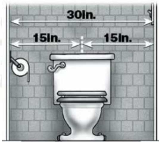
↑ toilet at east bathroom & master did not have required clearance
