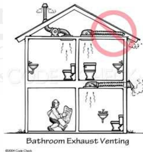
↑ unworkmanlike insulation; obstructing eave/soffit vents; also in this picture: exhaust fan(s) improperly terminate in the eaves, rather than to the exterior
