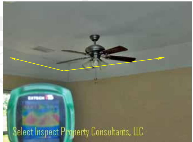
↑ Thermal imaging confirmed deficient insulation/venting
