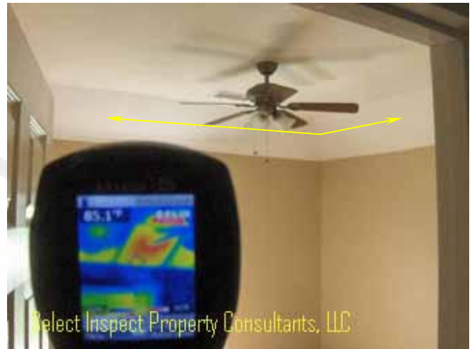
↑ Thermal imaging confirmed deficient insulation/venting
