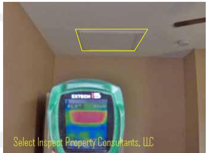
↑ Thermal imaging confirmed energy loss at the attic access
