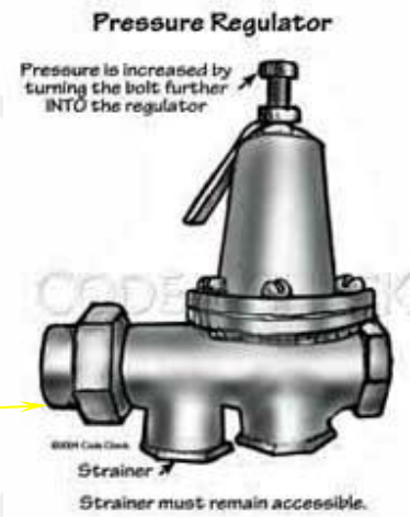
↑ pressure reducing valve had inadequate clearance from soil; Shut-off-valves require 3" clearance from soil
