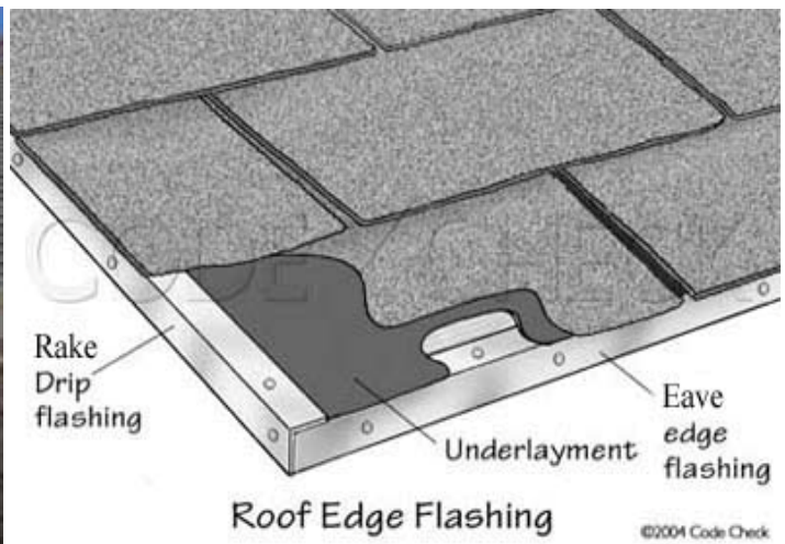
↑ example-unworkmanlike drip edge/felt; corners should have no gaps; rake (diagonal) edge & roof felt should be atop the eave (lower) edge flashing; roof underlayment should be under rake flashing. Also shown- metal protruding below shingle
