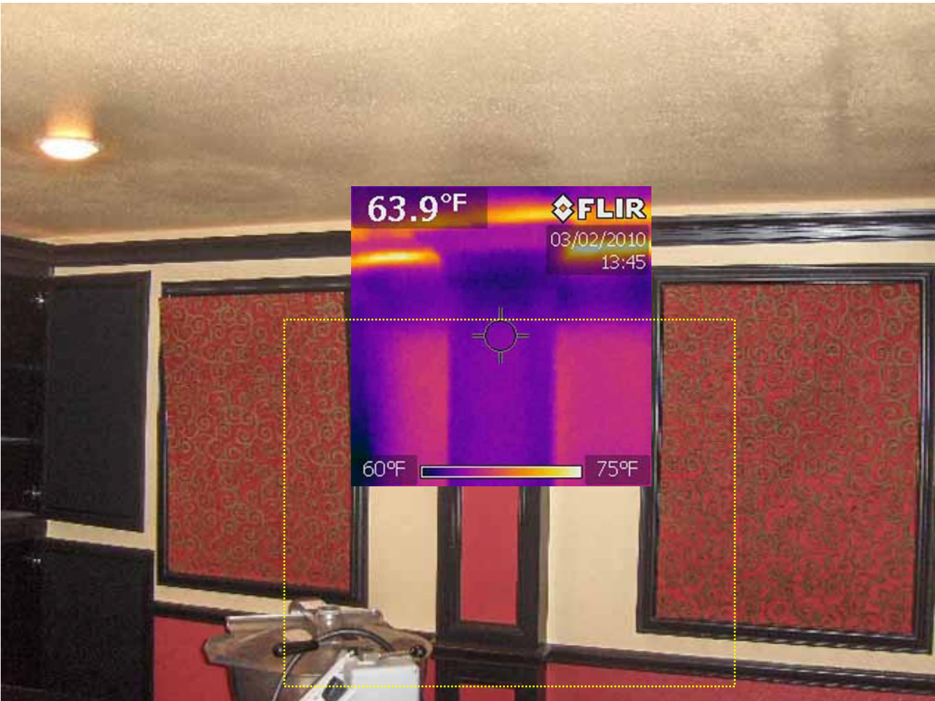
↑ inside adjacent the image above; abandoned window; energy loss
